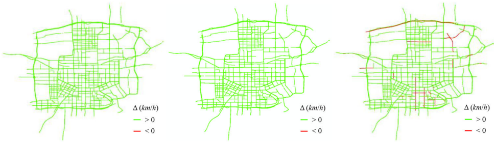
Figure 10. Comparison of the imputation errors of each road segment before and after introducing spatiotemporal correlations under the missing rate of 80%. (a) 1-month. (b) 1-week. (c) 1-day. Green indicates that the accuracy of data imputation has improved, and red indicates the opposite.
